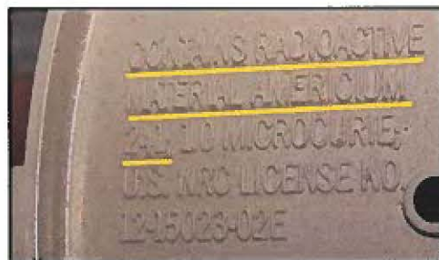
Radioactive material = Ionization or combo alarm
